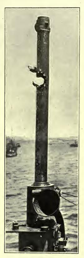
THE DAMAGED PERISCOPE OF THE SUBMARINE "EIL."
